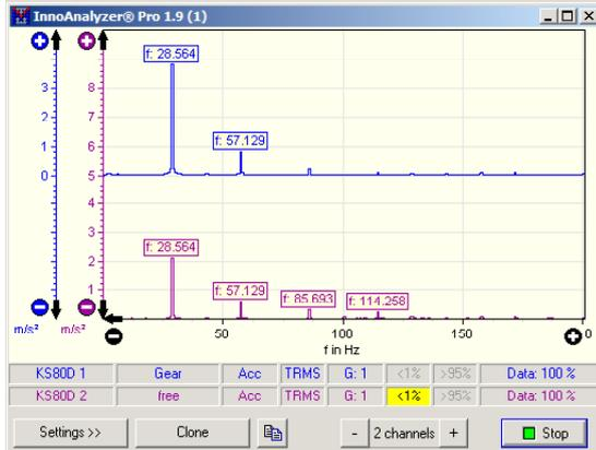
Simultaneous analysis of up to 4 signals, phase display switchable
