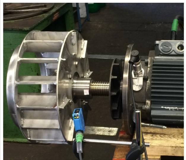
Pic. 1) Centrifugal fan mounted on the motor shaft.
