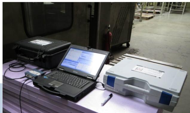
Pic. 2) With the VibroMatrix® system, you not only measure machine vibrations on site, you improve running smoothness on site through dynamic balancing in 1 and 2 planes.
