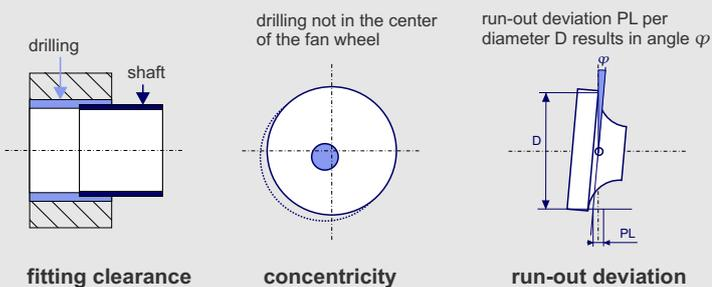
The individual imbalances of the impeller and drive motor resulting from the aforementioned influences add up vectorially to form a total imbalance during operation.
