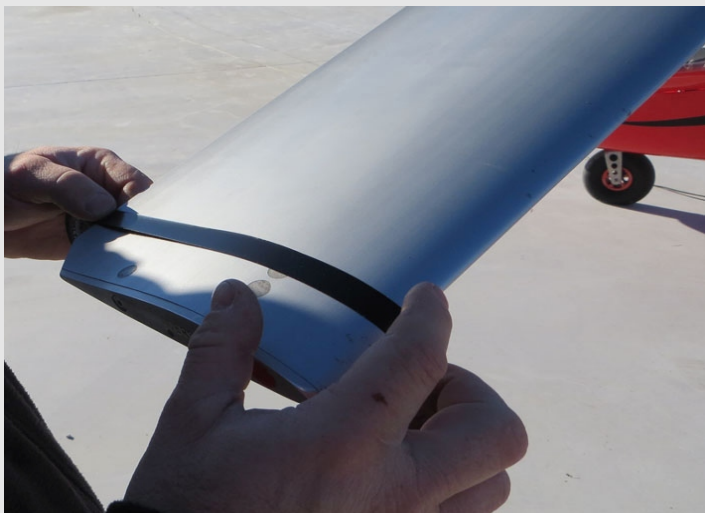
Putting a test weight (adhesive tape) on the rotor blade ...
