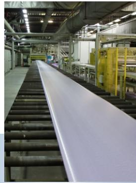
Product after the extruder, before the processing step face milling.
