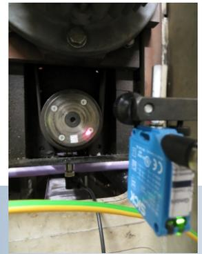
Vibration measurement on the bearing of the milling shaft and detection of the speed.
